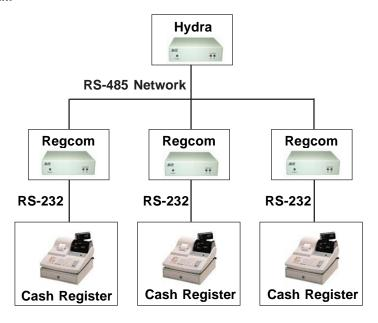
Figure 2C: Connection Diagram
